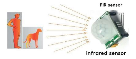
Infrared sensors measure the degree of Room ambient temperature with multiple detection beams and when detecting a difference At the temperature of a human body inside the detection area The sensor is activated, the lights Turn on, and when it leaves the body from the detection area range, the room temperature returns to what it was before Sensor activated and turn the lights off
