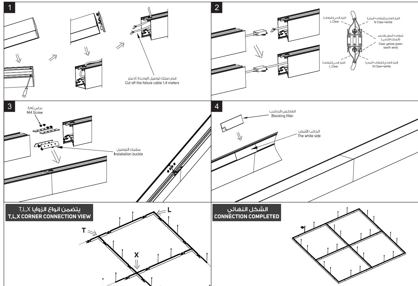
(1): Take out the end, then pull out the fixture cable, then cut off the cable, then connect the power cable to the fixture cable.
