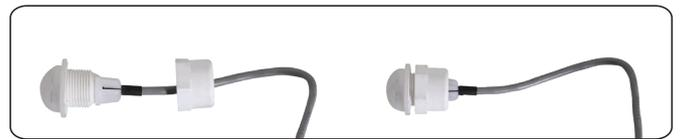
The nuts design at the head of the sensor makes it more convenient to fix on the installation object. There is also wiring for fixing made of plastic at its bottom in order to add its strength when being installed.
