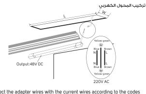
Connect the adapter wires with the current wires according to the codes attached to the product
