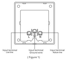
Connect the wires of the product with the screw product according to the symbols that are attached to the product.
