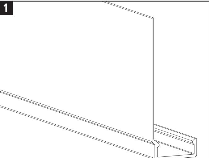
Cutting the suitable size and fix the flexible baffle by screws
