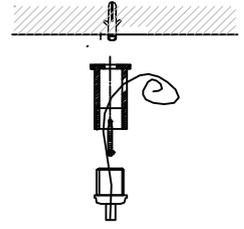
Fix the strain directly to the ceiling
