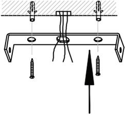
Fix the ceiling bracket to the ceiling
